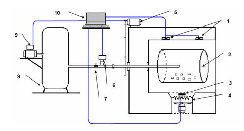
Fig. 1. Scheme of microwave-vacuum drying stand
