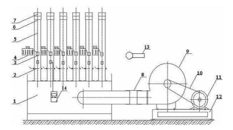
Fig. 2. Scheme of convection drying stand
