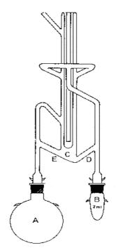
Fig. 3. Examining stand based on the Likens-Nickerson method
